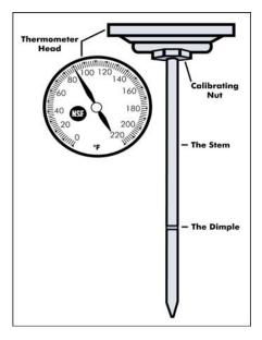
Metal-stem probe food thermometers with a temperature range of 0°F to 220°F are required to test food temperatures when holding foods hot, cold, or when cooking raw animal products. Clean and sanitize your thermometer using alcohol or sanitizing wipes after and before each use.
