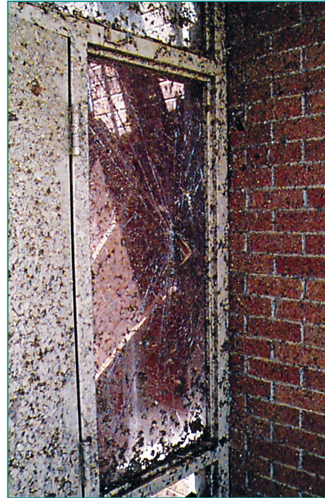
Figure 3-22 Impact performance of laminated glass. The corner of a table penetrated this laminated glass window, but the glass remained in its frame.
