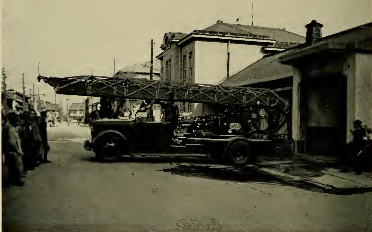
Above. Kyoto's aerial truck, located at Shimo battalion headquarters, equipped with 500 g. p. m. pump, but had no hose or standard ladder equipment.
