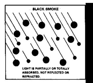
Figure 2-1. Action of smoke particles on light radiation.
