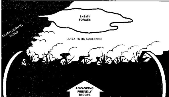
Figure 2-4. Screening smoke cloud for flank and quartering wind conditions.
