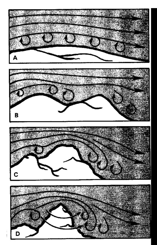
Figure C-10. Effects of terrain on wind.
