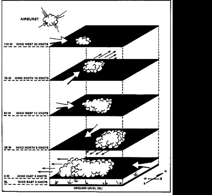
Figure C-9. Vertical wind distribution and its influence on the downwind hazard area at the surface (assumes inversion condition and little turbulence).
