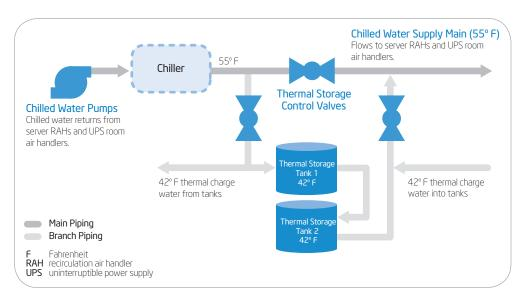
**Figure 2. Diagram of supplemental thermal storage system loop.** The valve on the main chilled water supply line is open during normal operation. In the event of an outage, this valve closes and the two valves on the thermal storage branch piping open to allow the water in the storage tanks to flow into the chilled water supply, providing cooling to the air handlers.
