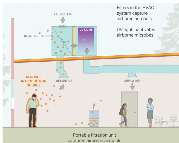
Figure 2: Sources of airborne aerosols and their infiltration
