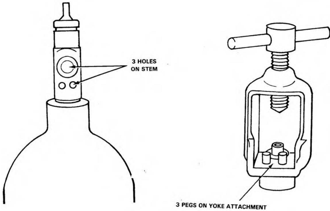
Figure 3-9. Cylinder stem and yoke attachment.
