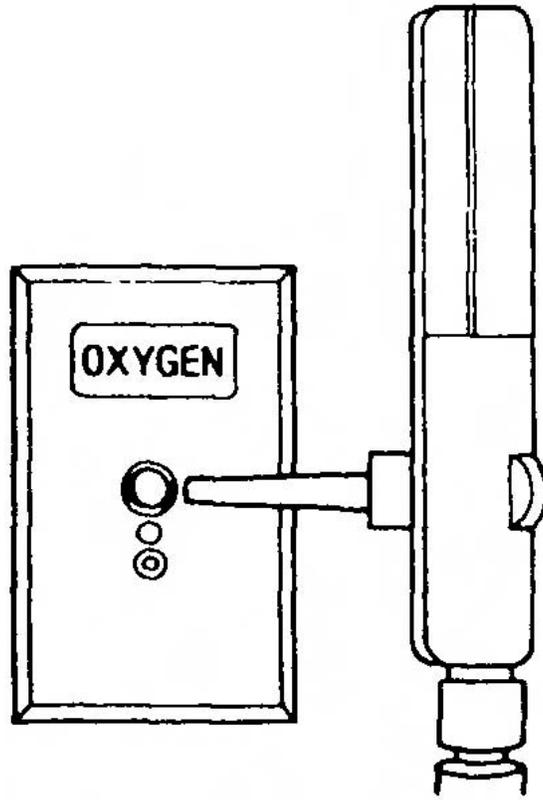
Figure 3-14. Attaching flow meter to "quick connect" coupler.
