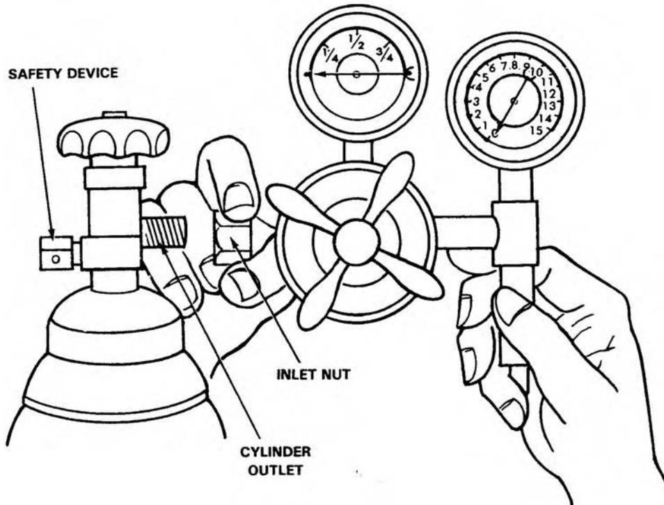
Figure 3-8. Attaching a cylinder regulator.
