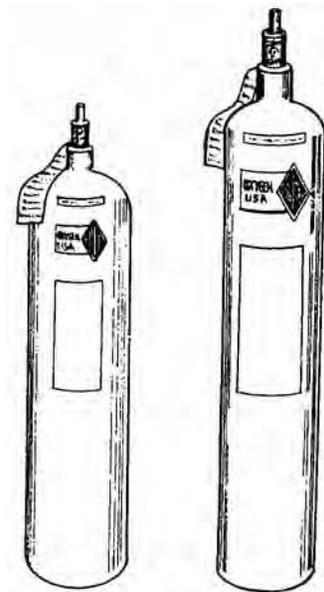
Figure 3-2. Oxygen (O<sub>2</sub>) cylinders.
