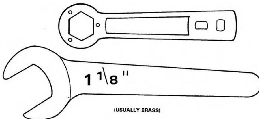
Figure 3-6. Nonsparking cylinder wrenches.
