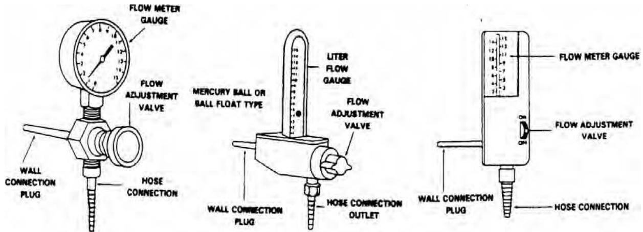
Figure 3-13. Flow meters for wall oxygen setups.
