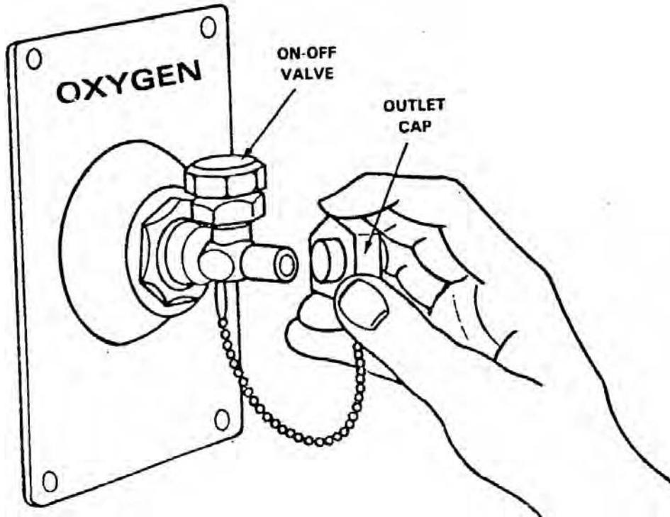
Figure 3-11. Manually operated valve.
