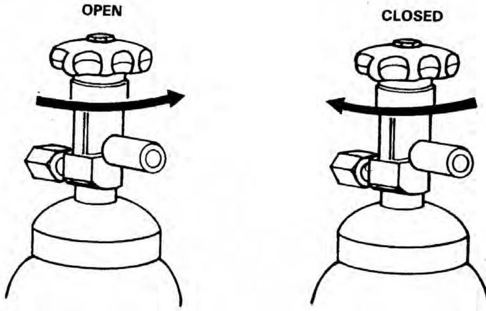
Figure 3-7. "Cracking" the cylinder.
