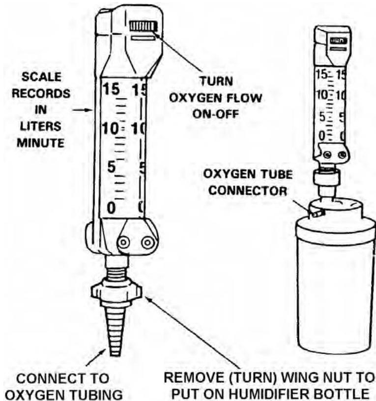
Figure 3-10. Attaching humidifier to flow meter.
