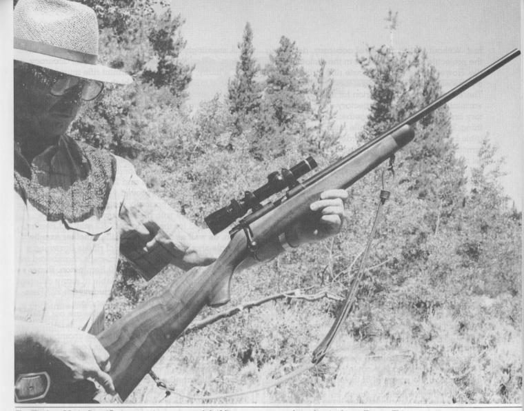
The Kimber 22-rimfire rifle is a semi-custom model of fine accuracy and mechanical excellence. This Kimber wears a Leupold 1.5X-5X variable scope sight for quick work on running rabbits, as well as longer shots.
