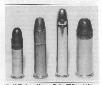
The 22 Winchester Magnum Rimfire (WMR) cartridge (second from right) is shown with a 32 Long rimfire (far right), an early attempt to boost rimfire power; the 22 Winchester Rim Fire (WRF), a round that fires a 45-grain bullet; and the 22 Long Rifle (far left). Note that the 22 WMR is the only one of the four that has a jacketed bullet.
