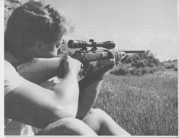
The Sako varmint rifle exhibits all the traits necessary for high-scoring: an accurate and heavy barrel, stiff action, good weight for steadiness, and chambering for a flat-shooting cartridge.
