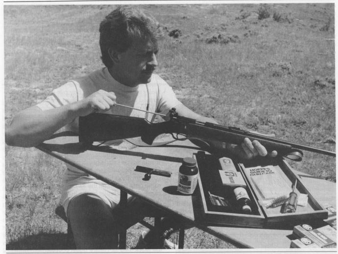
One rule of thumb to prevent damage from improper cleaning is to clean the firearm from the breech, not the muzzle, if at all possible.
