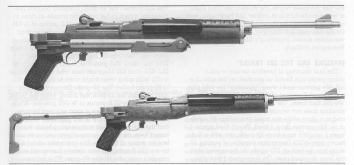
The 223 Remington has gained a great following due to its chambering in semi-automatic rifles such as the popular Ruger Mini-14. This versatile rifle is available in a folding stock model shown closed (above) and open (below).
