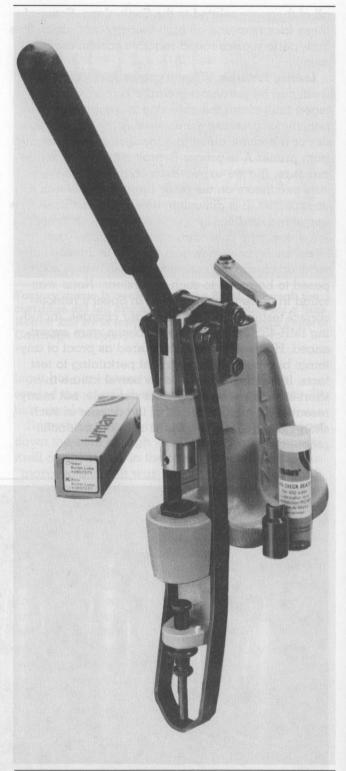
The Swift can be successfully loaded with cast projectiles. This bullet sizer with lubricator is used to ensure proper dimension of the projectile.
