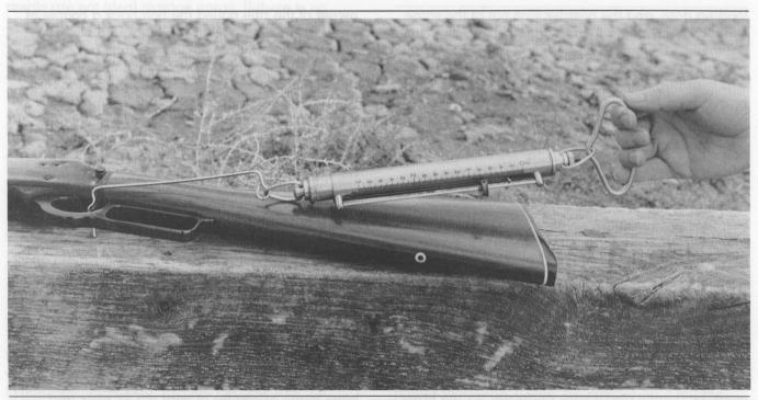
Check your trigger pull or have it checked by a gunsmith, but do not alter triggers yourself unless you are duly qualified. The job of altering trigger pull is best left to an expert.
