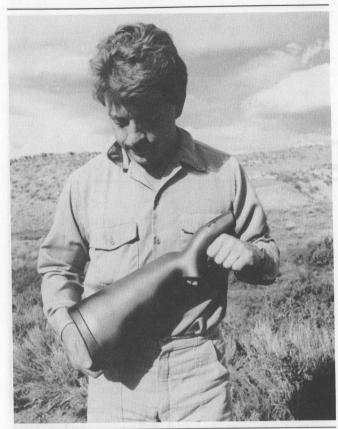
The Charter Arms AR-7 rifle is a prime example of the survival gun. Here it is shown in its own floating case, which is the buttstock of the rifle.
