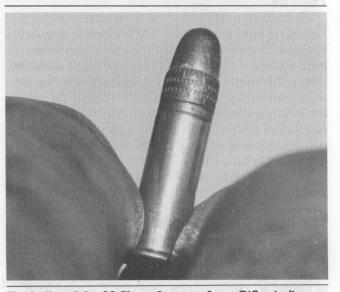
The bullet of the 22 Short, Long, or Long Rifle rimfire cartridge is the same diameter as the body of the case. Therefore, the base of the projectile must be reduced in size in order to fit into the mouth of the cartridge.
