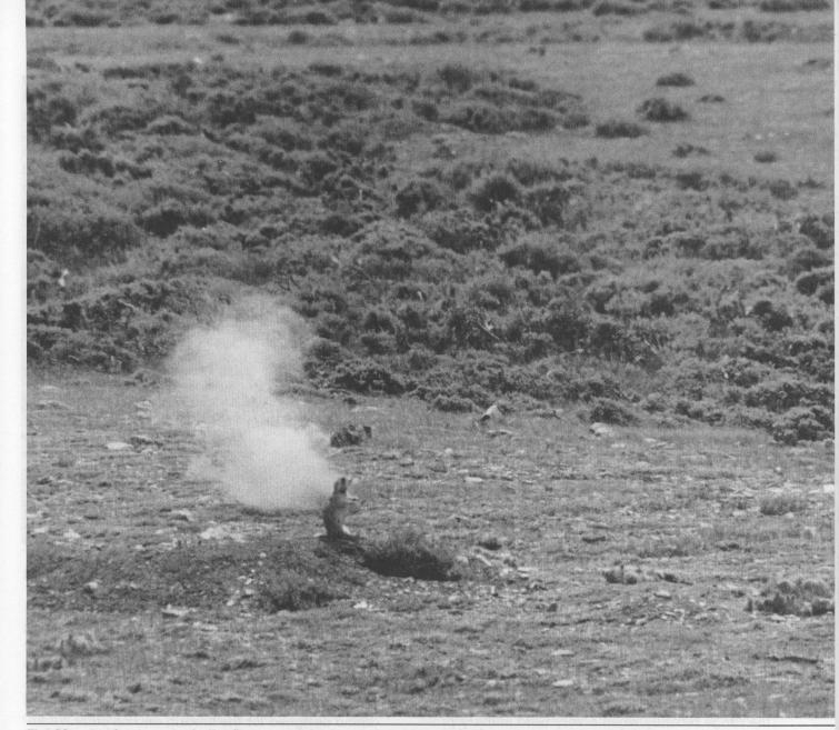
The 22-centerfire varmint bullet flies at such high speed and is so lightly constructed that it generally explodes upon contact with the ground, as shown here. The bullet missed the prairie dog, but it did not ricochet from the hard ground—it fragmented.
