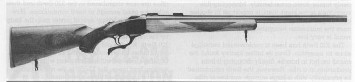
Many different rifle styles have been chambered for the Swift, including the single-shot Ruger No. 1 Special Varmint with 26-inch barrel.
