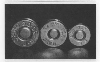
The 22 PPC USA cartridge (center) has a head size in between the 30-06 and the 222 Remington.
