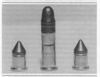
Rimfire cartridges carry priming mixture located around the rim of the cartridge, hence their name. The 22 Long Rifle rimfire cartridge, center, is flanked by two 22 CB Cap cartridges.
