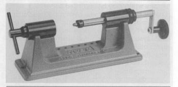
Because case stretch is prominent in "hot" cartridges, this case trimmer becomes an important tool for tailoring any centerfire cartridge, including the Swift, with maximum loads.
