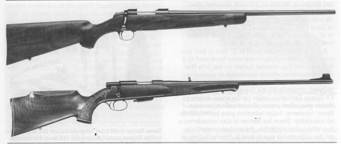
The 22 Hornet is currently chambered in some of the finest rifles of any era, including the excellent Kimber (above) and the Anschutz Model 1432 rifle (below). The small cartridge allows a petite rifle built around a short action.
