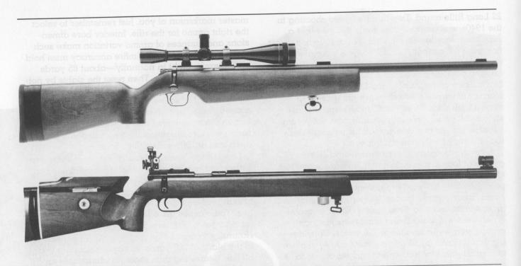
Two-hundred-yard shooting is enhanced with a rifle like the one above, built for stability, and wearing a powerful telescopic sight. Iron sights also work well for 200-yard rimfire shooting, especially when they are micrometer aperture sights mounted on a fine target rifle such as this Anschutz 1411 (below).
