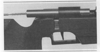
The use of a bore guide ensures that the cleaning rod will not lap the chamber area. Shown is a special bore guide designed for the 22-rimfire rifle.
