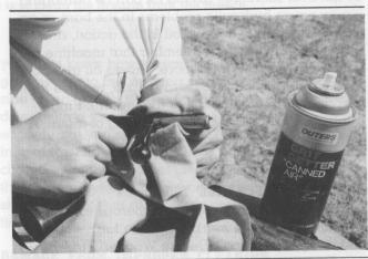
The bolt of the rifle is wiped down with solvent, then lightly oiled for preservation and prevention of friction. A film of oil or grease allows the bolt to work more freely.
