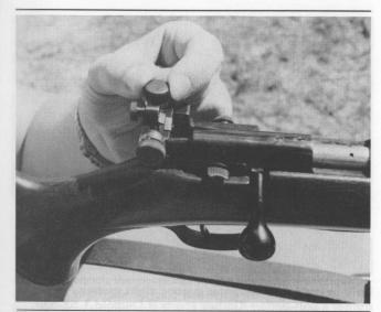
In sighting the micrometer "peep" rear sight, click adjustments are used. Each click has a definite value at the target in terms of minutes of angle.
