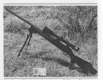
The Harris Bipod greatly enhances field steadiness. These bipods attach to the rifle and can be swung into place swiftly. Some models work from the sitting as well as prone position. This Harris bipod has been installed on a 22-250 rifle.
