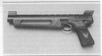
Browning's Buck Mark 22 pistol in the silhouette model offers a 9<sup>7</sup>/<sub>8</sub>-inch barrel with a .900-inch muzzle diameter. Precision sights include a Millet Gold Cup No. 360 with interchangeable front posts.
