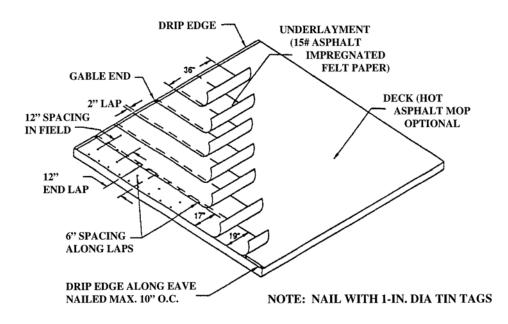
□ Select a high wind rated roof covering and, regardless of type, ensure that it is installed in accordance with the manufacturer's recommendations for high wind regions.
