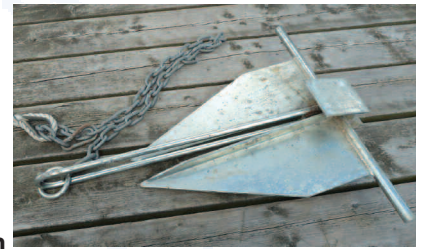
Danforth anchor with chain and shackle
