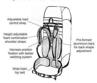
Figure 2.7: An example of a harness system
