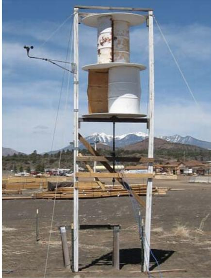
**Figure 8: Double step Savonius rotor**
