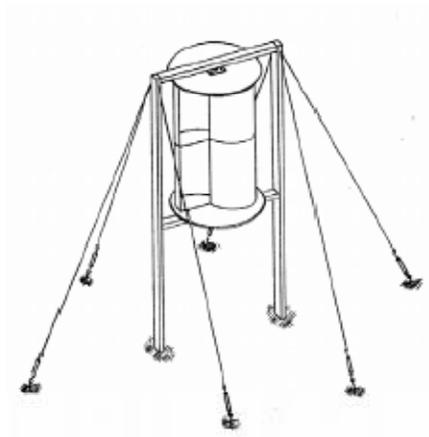
Figure 1: A practical Savonius windmill and tower (Brace Research Institute, 1973).
