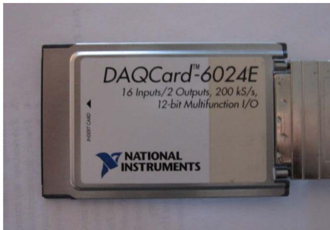
**Figure 19: NI 6024E Data Acquisition Card**
