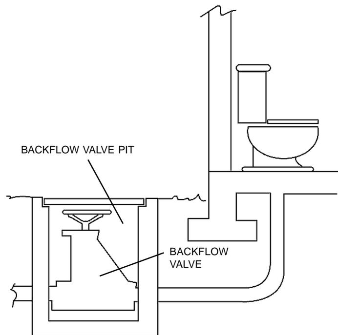
← NORMAL DIRECTION OF FLOW (VALVE PREVENTS FLOW IN REVERSE DIRECTION)
