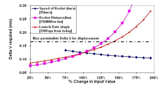
Figure 6: Sensitivity analysis of various decision parameters on  $\Delta V$  required for deflecting the asteroid from earth impact orbit
