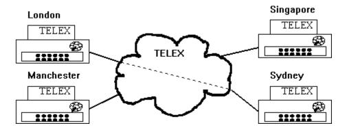
FIG 3 The international TELEXTELEX system is the text version of the PSTN. Any TELEX can 'dial' any other telex and leave a message even if the receiving machine is unattended.
